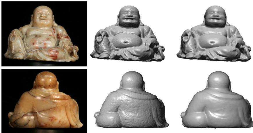
**Fig. 15 Reconstructing coloured jade.** Left: Two input images. Middle: model obtained by multi-view stereo method from [17]. Right: proposed method. The resulting surface is filtered from noise while new high frequency geometry is revealed (note the reconstructed surface cracks in the middle of the figurine's back).
