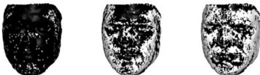
**Fig. 8** Distribution of inliers (in white) for  $\tau = 2$ . From left to right: 3 pt algorithm, 4 pt algorithm, Phong model. Note that the greasy forehead is classified as an outlier (black) in both 3 pt and 4 pt algorithms. After optimization of the Phong model parameters, the forehead points fall within the inlier threshold
