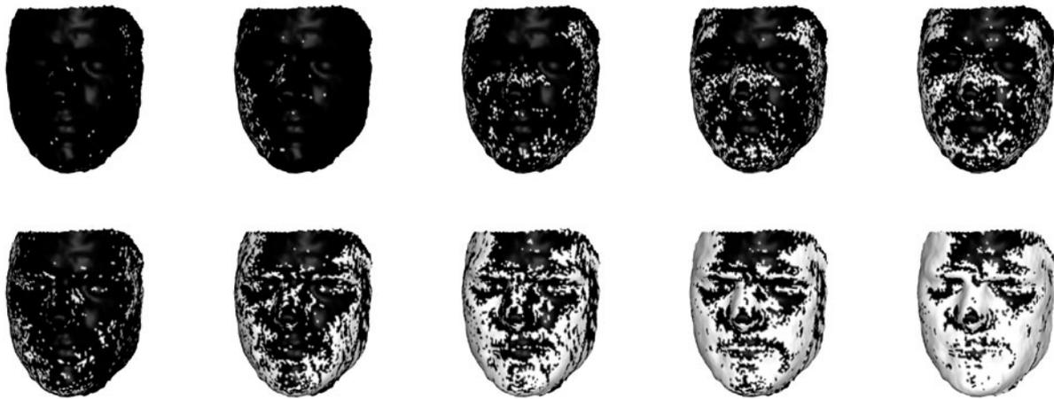
**Fig. 7** Distribution of inliers (in white) as a function of the threshold  $\tau$ . From left to right,  $\tau = 1, \tau = 2, \tau = 3, \tau = 4, \tau = 5$ . The image intensities are quantized in the range from 0 to 255. The *first row* shows
