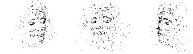
**Fig. 14** Sparse set of 3d points after using a structure-from-motion algorithm on the sequence of Fig. 9. From left to right, the 3d points are shown from three different viewpoints roughly at  $-45$  degrees,  $0$  degrees, and  $45$  degrees
