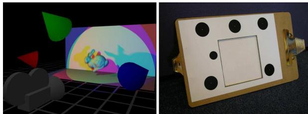
Figure 1. **Setup and calibration board.** Left: a schematic representation of our multispectral setup. Right: Linking the two clipboards and attaching a printed calibration pattern produces a planar trackable target for computing the orientation of the pattern's plane. Cloth inserted between the boards appears in the square hole and creates the association between color and orientation.
